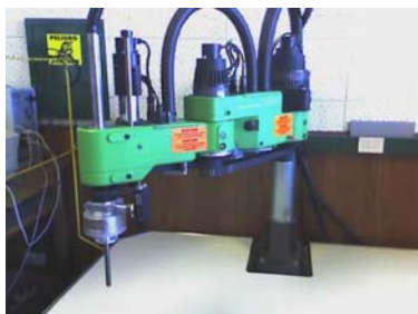
Fig. 1. Robot industrial Bosch SR 800.
